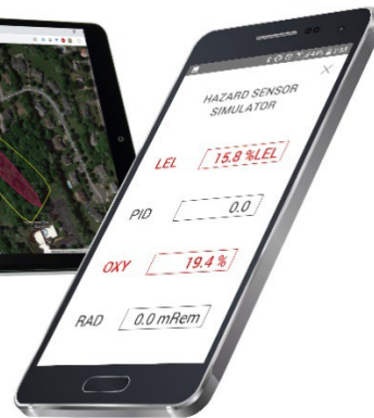
SensorSim with I-Phone sensor simulator and GPS-based hazard simulator
